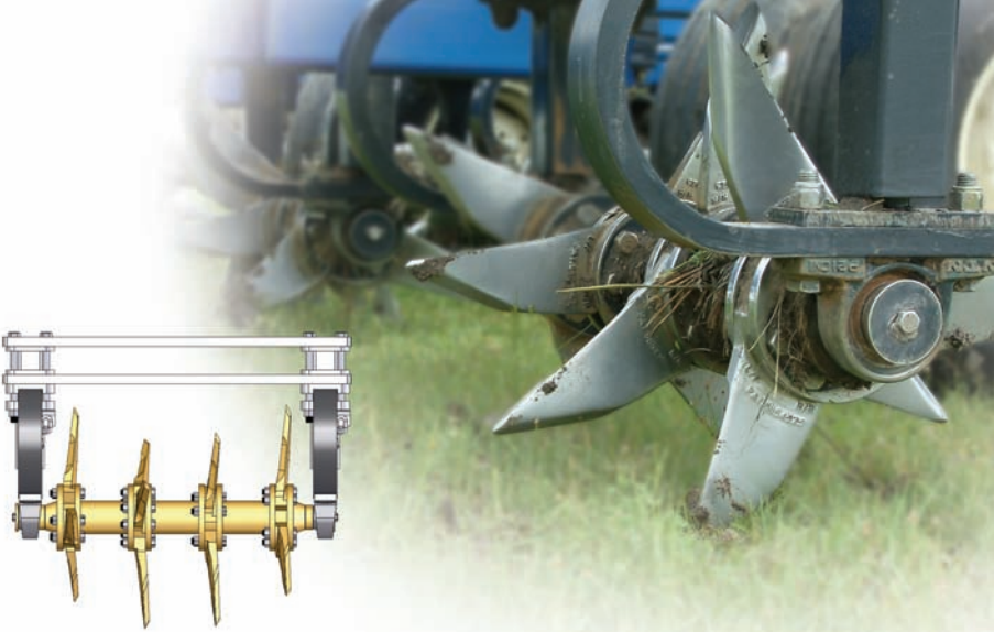
Closeup of the distinctive design of Smart-Till's tines
